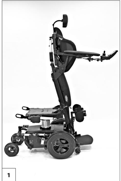
The stand up process [1] can be adjusted with the control module.
